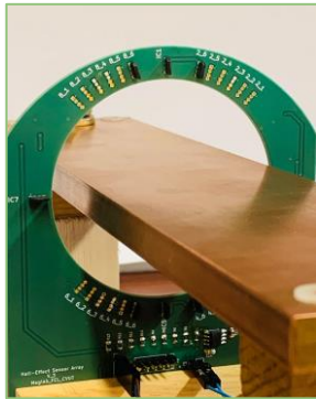
Fig. 17. The prototype of the improved circular array-based current transducer for rectangular busbar.
